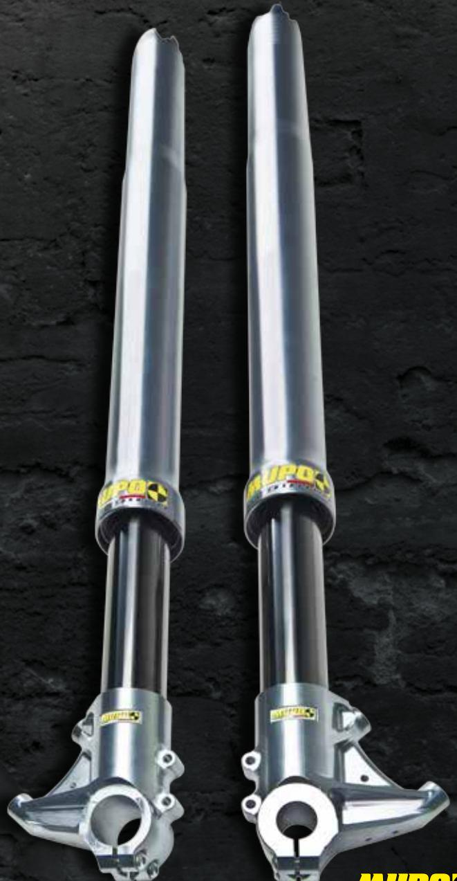
The fork, with stanchion tubes of 38 mm in diameter, is adjustable in compression, rebound and spring preload.
